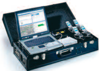
R&S Suitcase: GSM/UMTS/CDMA2000 Scanner, 4x mobiles, GPS, QoS (Network-Qual., Data Qual., Speech Qual. PESQ-MOS)
